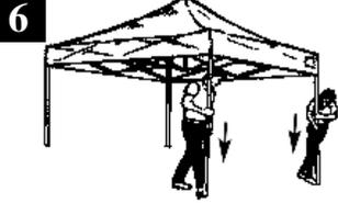
**6** Adjust the legs to the desired height by stepping on the footpad and lifting the leg up until it clicks into place. Repeat for each leg. There are multiple height adjustments that can be made by pressing the release lever and lifting the leg until the next click.
