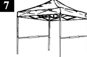
**7** Optional Side Rail hardware consists of 3 metal bars that fit together to form a 10' span. Simply assemble the bars, slide the fabric skirt over the bar, and clamp the bar to the frame using the included bar clamps.
