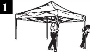
**1** Press the lever on the leg bracket to release the locking pin and slide the inner leg up. Repeat on the other 3 legs.
